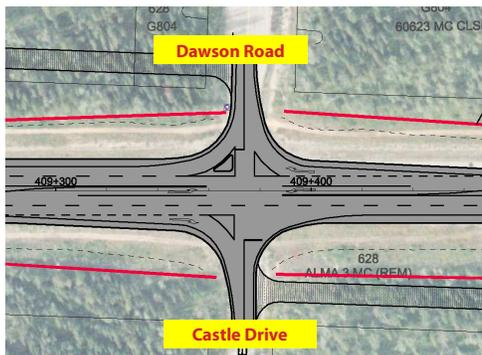
*The drawings shows constructed and painted islands. **Specific provision for pedestrian crossing of the highway has not been made at Dawson Road.** During the next design phase, an assessment will be made of existing pedestrian volumes and requirements for pedestrian connectivity in the area to determine the warrants for a pedestrian crossing at this location. The assessment will be made in accordance with guidelines developed for the Yukon Government.*
